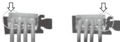
Wrong (1) Not enough cover insertion. Wrong (2) Not enough cover insertion.
